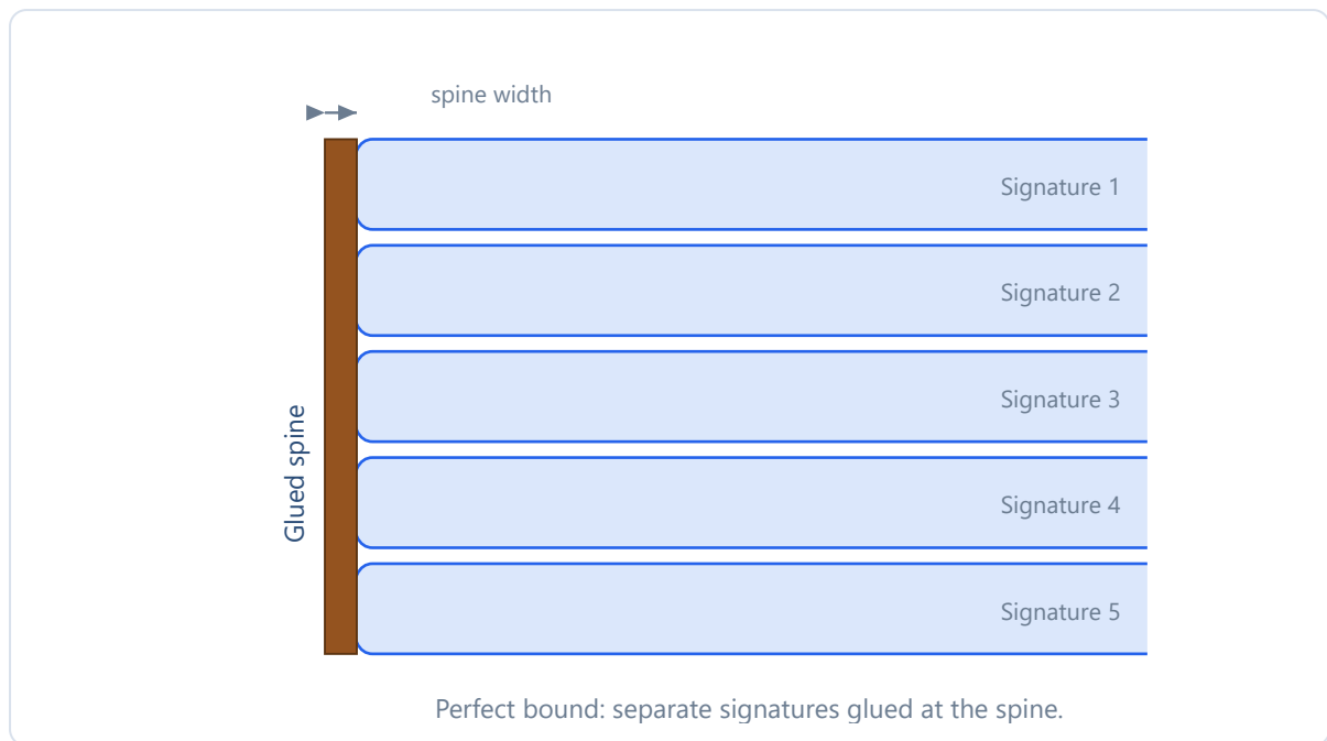
Fig. Perfect binding: stack of signatures and the spine.
